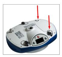
• Keeping one hand on the battery still in its compartment, put the ProMark 500 the right way up. The battery will then easily slide out of the battery compartment.
